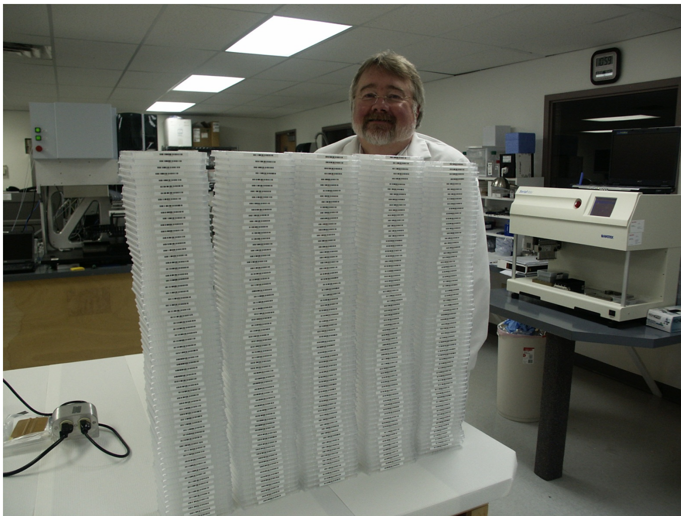
300 384-well plates run on Roche LightCycler 480 in ~60 days with 10ul reactions
